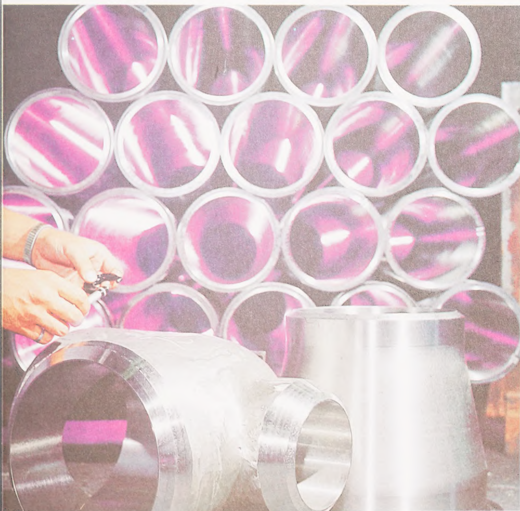
Products of the F-W centrifugal casting process. High-integrity vertically cast fittings for use in the petrochemical industry are shown against a backdrop of horizontally cast stainless steel lattice tubes used in nuclear reactors.
